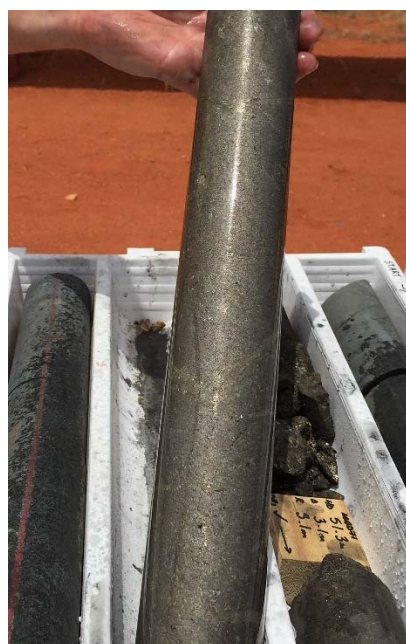
Figure 1 - drill core from the 17.45m high-grade intersection in MAD71. The section of drill core shown is from the massive sulphide interval that returned assays of 2.02m @ 5.05%Ni, 2.01%Cu, 0.21%Co and 3.31g/t total PGEs from 50.6m
