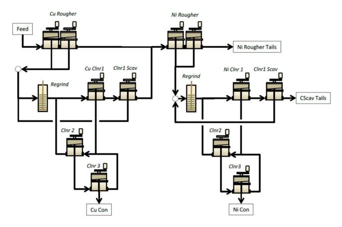
Figure 1: Flowsheet for sequential flotation used for metallurgical results in this report.
