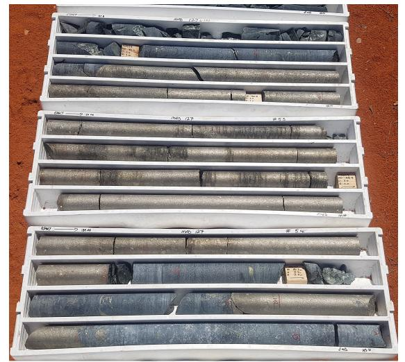
Figure 2 – photo of drill core tray for MAD127 showing the massive sulphide interval from 183.9m downhole
