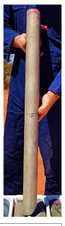
Figure 1 (above) - photo of drill core from MAD136 at Investigators which intersected over 20m of mineralised ultramafic; core shown is massive sulphides between 149.55m to 151.93m with average XRF readings of 8.1%Ni and 3.21%Cu (assays pending) – see ASX Release dated 30 November 2018 'Assays Confirm Best Ever Intercepts at Mt Alexander'
