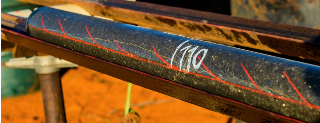
Figure 2 – drill core from MAD166 with massive sulphides at 110m downhole.
