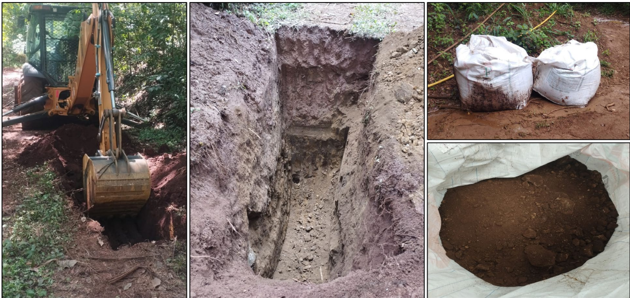
Figure 4 – Trench sampling of near surface saprolite mineralisation, providing approximately 5 tonnes of representative material for metallurgical testwork.
