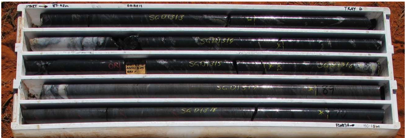
Figure 1 – Core (wet) from DDD011 that contains the Zn-Cu mineralised zone. The metal-rich sulphide bands are visible in the core.
