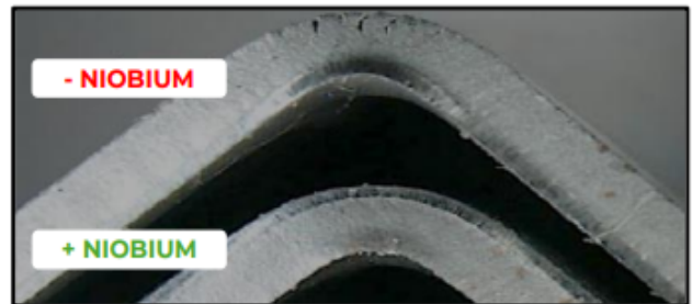
Figure 20: Improved microstructure of steel with Nb additions Figure 21: Improved flat sheet formability with Nb
