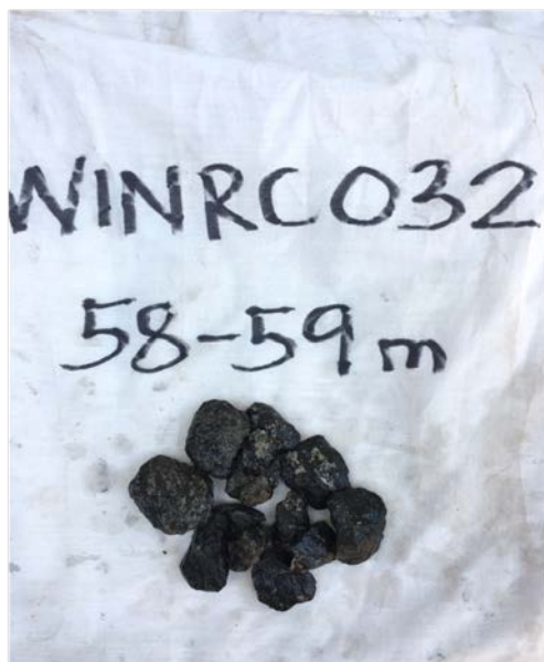
Figure 5 – a sample of the drill chips from WINRC032 which exhibit strong hydrothermal alteration and sulphide mineralisation, which may have a gold association.
