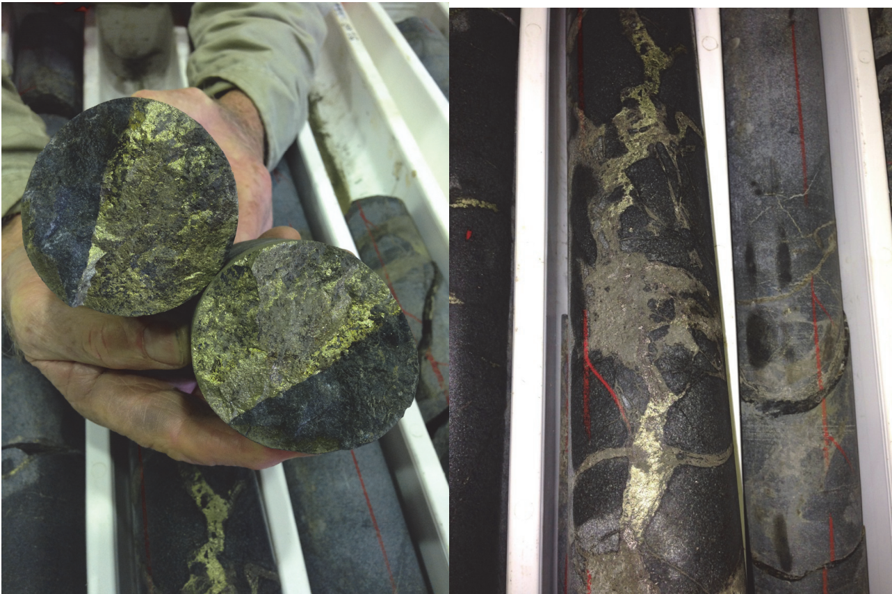
Figure 3 – on left: drill core from MAD22 with massive chalcopyrite (yellow-green) in contact with ultramafic (dark grey) from 52.4m to 52.63m with 13.1%Cu and 43g/tAg. on right: drill core from MAD22 (50.26 to 50.8m) showing nickel-copper stringers (the light yellow is chalcopyrite and the tan brown is pentlandite-pyrrhotite). These stringers likely remobilised from massive sulphides that may be the off-hole DHEM conductors near MAD22.
