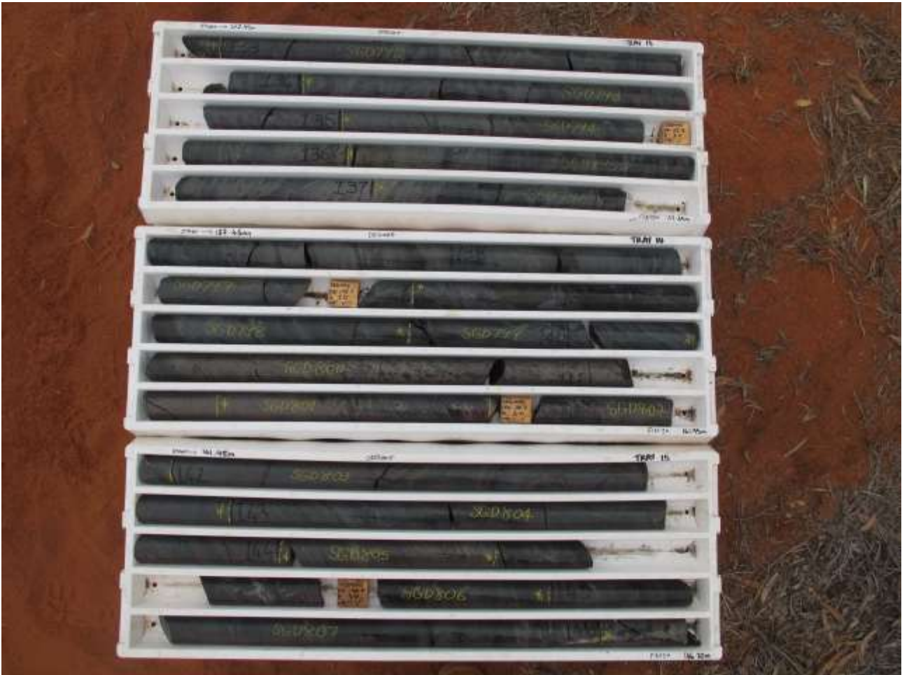
Figure 3 – Sections of drill core from DDD005. Section SGD800, amongst others, clearly shows massive brecciated sulphidic units.
